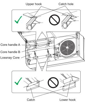
Check that the louver is closed and close the panel. (If the louver is open, the panel may get damaged.)
