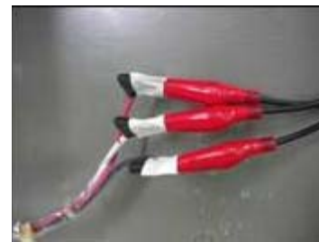
Fig. 2-4 Clip covered with insulation tape
