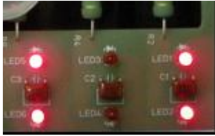
Fig. 2-12 LED indication when V phase is open.
