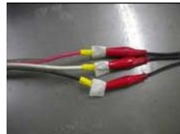
Fig. 2-7 Clip covered with insulation tape
