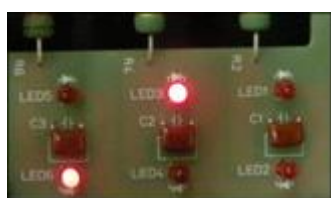
Fig. 2-10 Example of LED indication in compressor protection control (Do not conclude your fault identification at this stage.)
