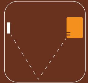
Fig. 4 On the wall, opposite to the indoor unit
